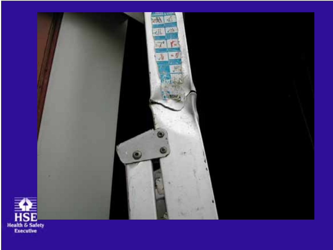
Split stile – Class 1 industrial steps. Beyond repair
