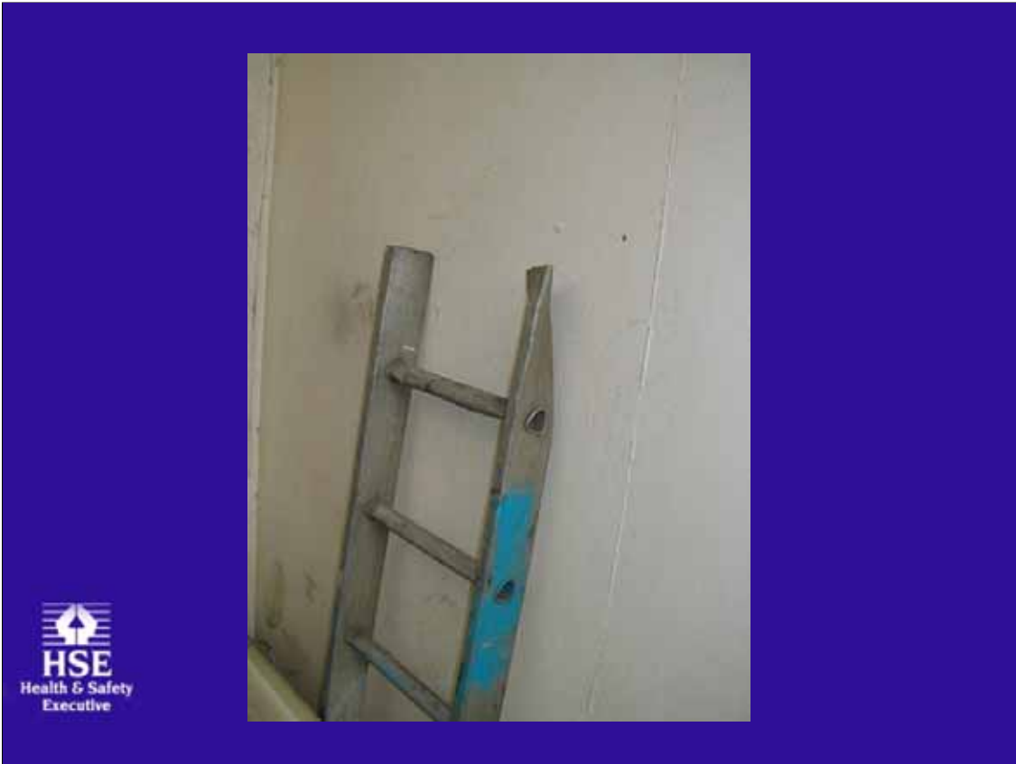
Twisted stile – beyond repair
