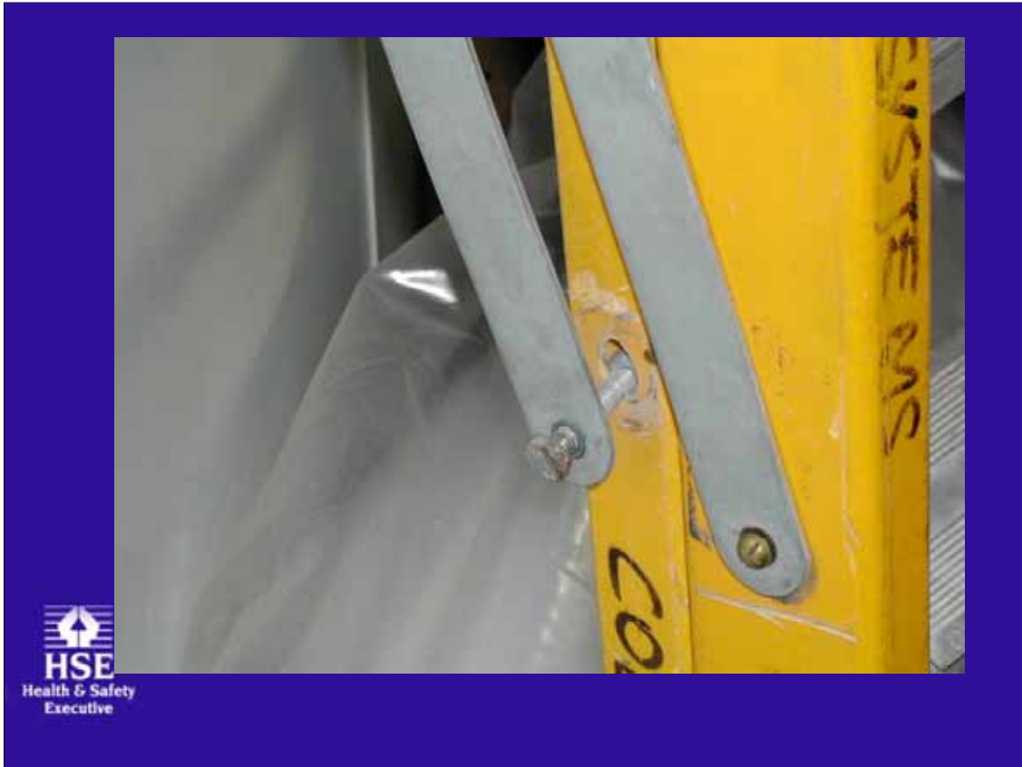
Damaged restraint connection – Beyond repair hole in stile has been worn or made larger
