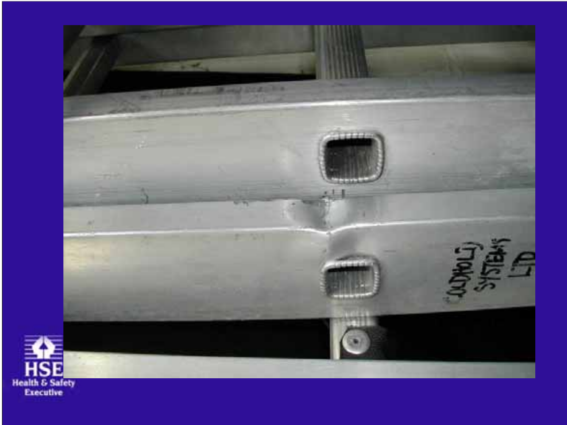
Dent in stiles – Beyond repair
